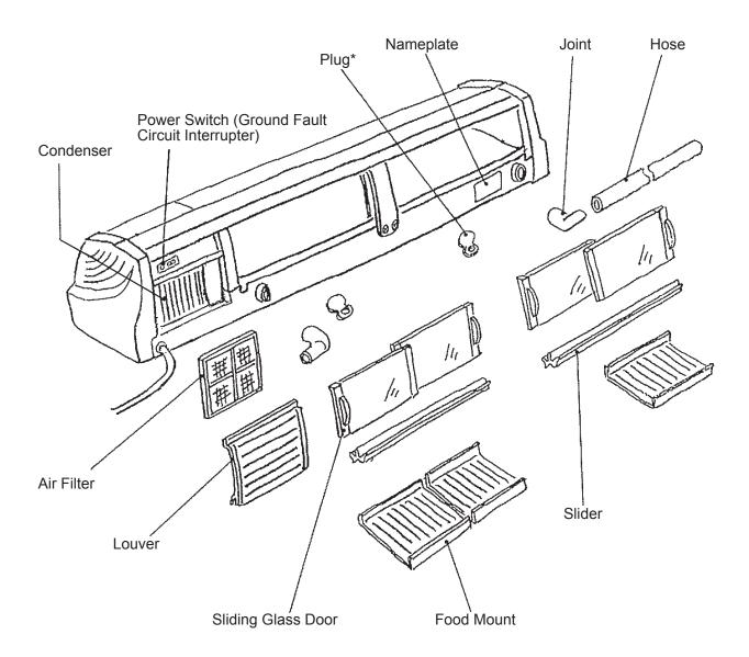
\*Note: Always attach the plug(s) to the drain holes located in the showcase.
